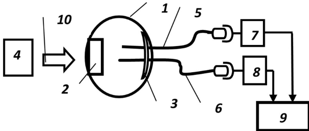
Figure 2. Scheme of the experiment, consisting of a YAG laser, an eye, a system for fixing laser radiation (two optical fibers), two photodetectors and an oscilloscope: 1 - eyeball; 2 - posterior capsule of the lens; 3 - retina; 4 - YAG laser Yatagan-4M; 5, 6 – multimode optical fibers «pigtaills» FC 62.5 / 125; 7, 8 - high-speed photodetectors; 9 - digital oscilloscope GDS-71102A; 10 - a stream of laser radiation
