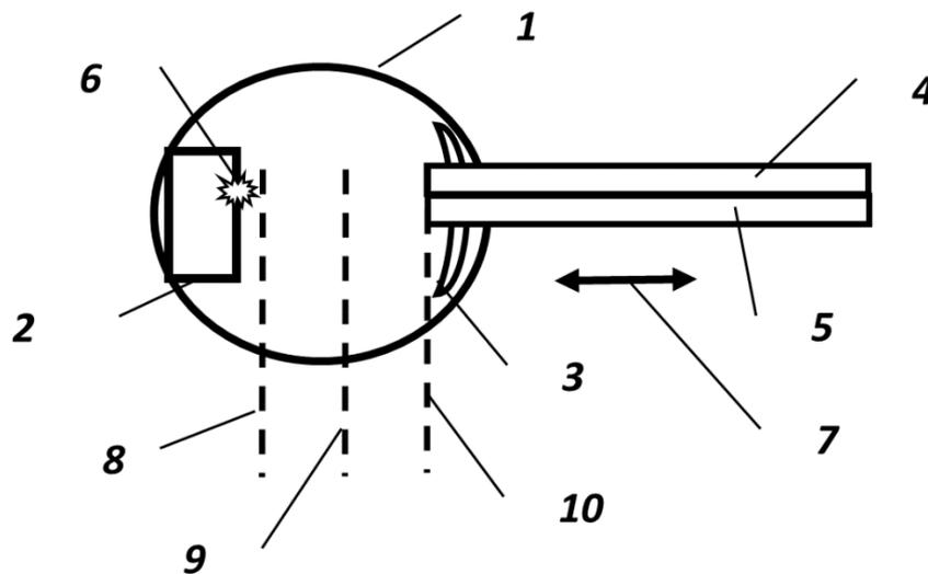
Figure 3. Scheme of the optical fibers position inside the eye: 1 - eye; 2 – lens capsule; 3 - retina; 4, 5, - optic fiber; 6 - area of action of laser radiation; 7 - direction of displacement of the distal ends of the optical fibers; 8, 9, 10 - the positions of the distal ends of the optical fibers: "behind the posterior capsule", "in the middle of the vitreous body" and "near the retina" in the region of the posterior pole of the eye
