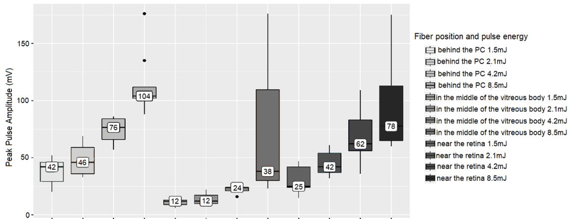
Figure 4. The amplitude of the pulse depending on its energy and the position of the fiber inside the eye
