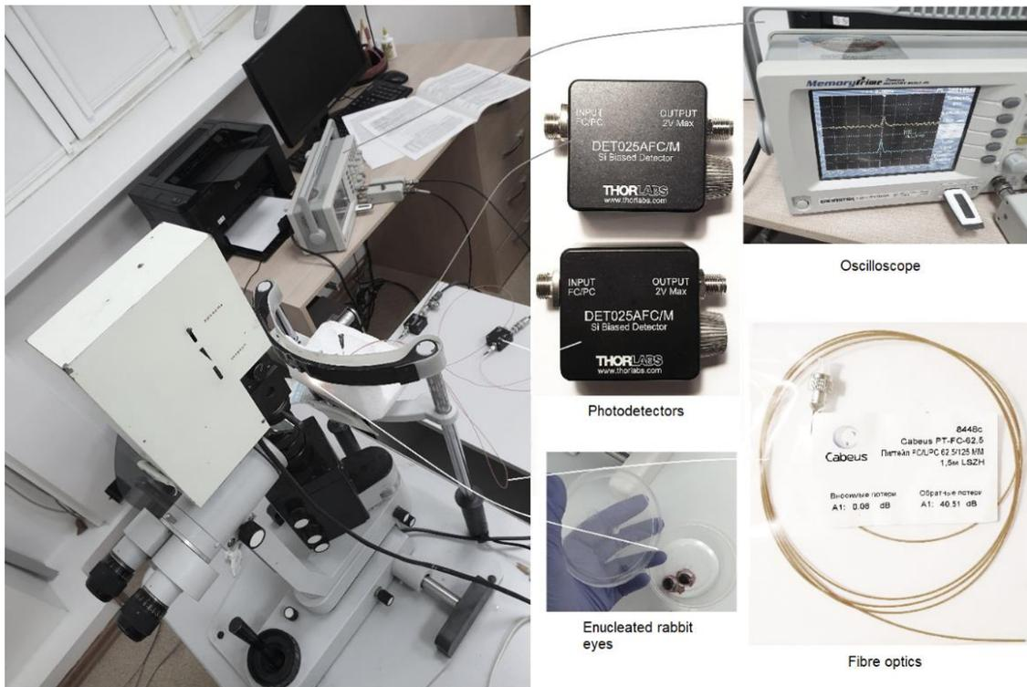
Figure 1: Photograph of the experimental model, consisting of a YAG laser, an eyeball and a laser power measurement system (two optical fibers, two photodetectors and two-channel oscilloscope)
